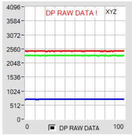
In order to understand with which **X**, **Y** and **Z** values the sensor works in parameter set 2, you can display this raw data in the display **XYZ** using the **DP RAW DATA** check box.
