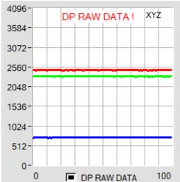
In order to understand with which **X**, **Y** and **Z** values the sensor works in parameter set 2, you can display this raw data in the display **XYZ** using the **DP RAW DATA** check box.
