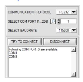
A click on the magnifier symbol in the **CONNECT** tab opens a list with all the possible **COM PORTS** in the display.
